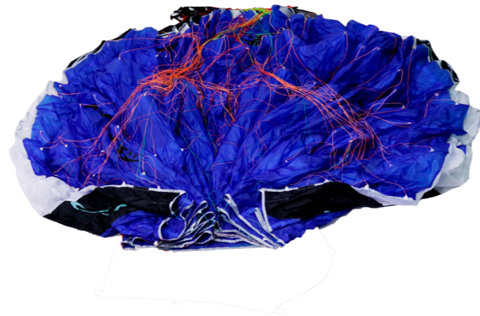
Step 2: Begin with the center of the trailing edge. Put one profile over the other. Each side separate.
